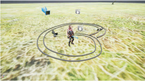
Figure 8: The guide rail and the cameras focused on the meta-human, our in-environment character. The main character is placed on the virtual ground floor. A cinematic camera was attached to the guide rails to capture the overall view of the scene while the focus of the subject was the main character, the meta human. The camera was a child of the parent guide rail.
